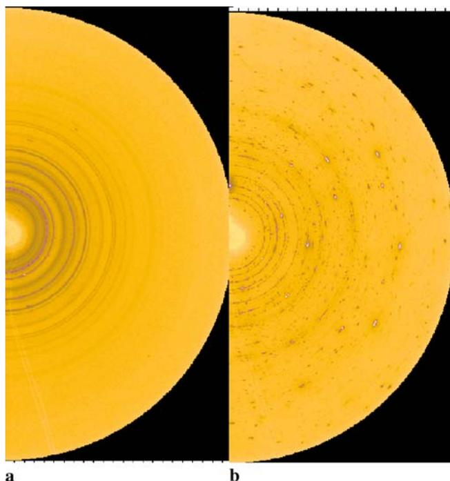
**FIGURE 5** Synchrotron X-ray diffraction patterns (half of image plate) for the bronze vessel fragment at (a) region near the corner ( $100 \mu\text{m}$ ), where only the diffraction rings from the corrosion layer (a combination of cuprite and cassiterite) are present and (b) the bulk ( $1040 \mu\text{m}$ ) where diffraction spots for the bronze phases (copper, tin-rich, and lead phases) are visible, together with faint corrosion phase rings
