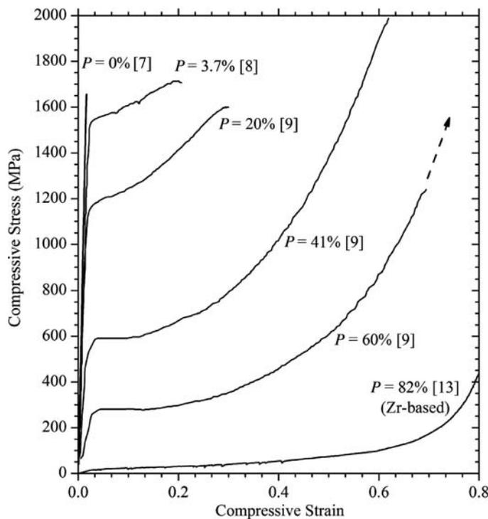
Figure 3. Compressive engineering stress–strain curves for several porous amorphous metals at intervals of approximately 20% porosity  $P$ . All but the highest-porosity material (which was processed from  $Zr_{57}Nb_5Cu_{15.4}Ni_{12.6}Al_{10}$ ) were processed from  $Pd_{42.5}Cu_{30}Ni_{7.5}P_{20}$ .
